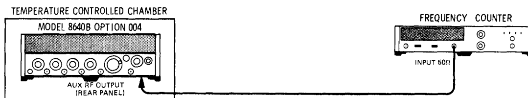
Figure 4-2. Frequency Stability vs Temperature Test Setup
